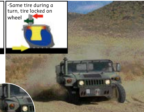
\ HMMWV equipped with Hutchinson VFI™ with integrated Beadlock
