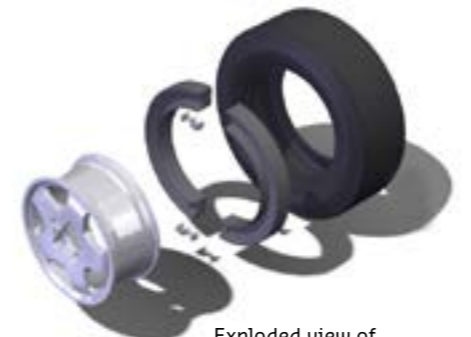
Exploded view of a wheel/tire/CRF assembly
