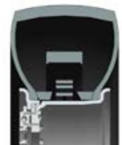
Cross section of a CRF mounted on a wheel
