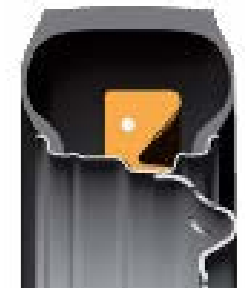
Cross section of a CRF mounted on a wheel
