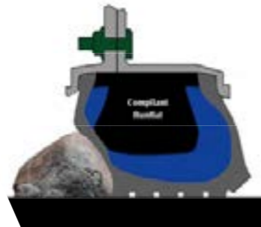
The compliant system does not damage the tire
