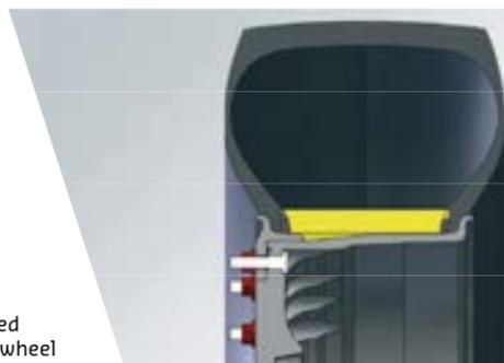
Hutchinson Beadlock mounted on a 2 piece bolted together wheel
