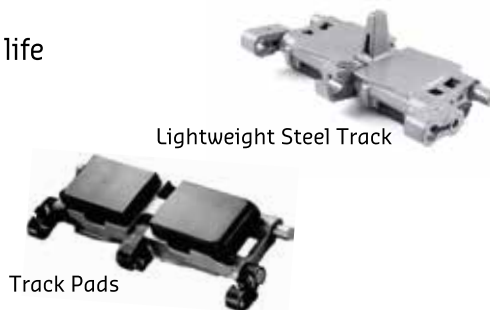
Replaceable Track Pad without screws or bolts
